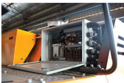
Separate fuse and controller box
