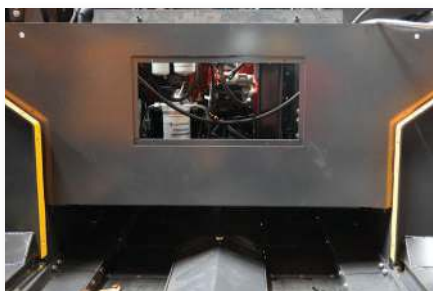
Remote engine oil filter for easy access
