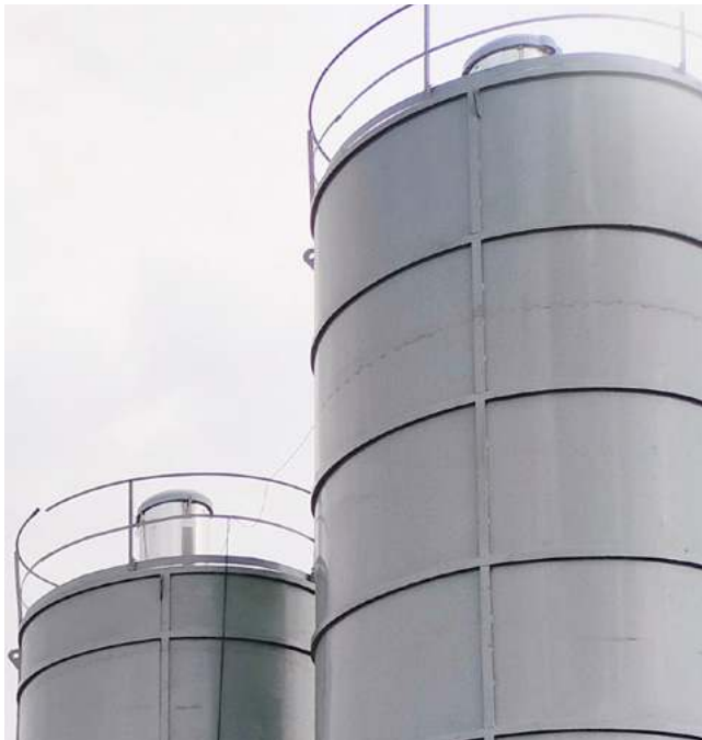
Top Mounted Dust Collector
